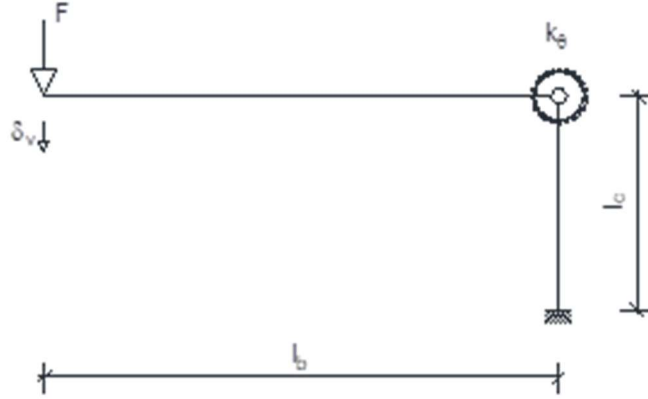
Figure 75. Rotational spring for evaluating the adhesive layer deformability.
