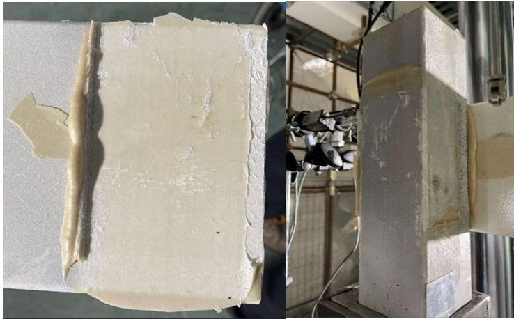
Figure 61. Cohesive failure (in the adhesive mainly) for the joint configuration of Group A.4.
