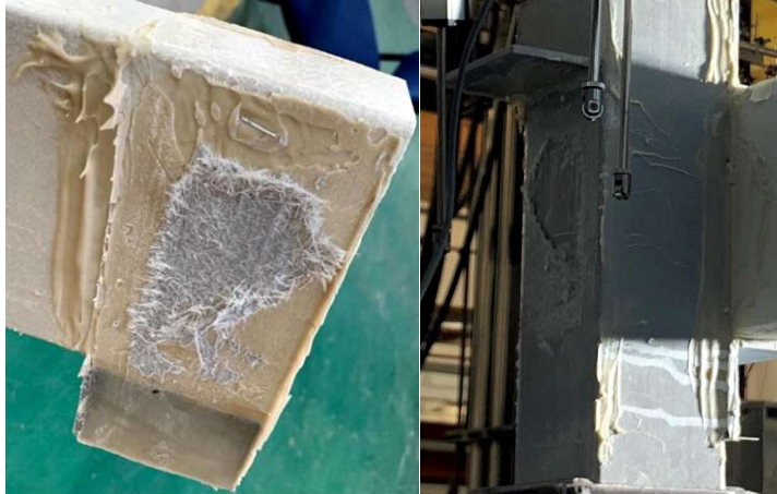
Figure 57. Mixed failure between resin and GFRP for the joint configuration of Group A.1.
