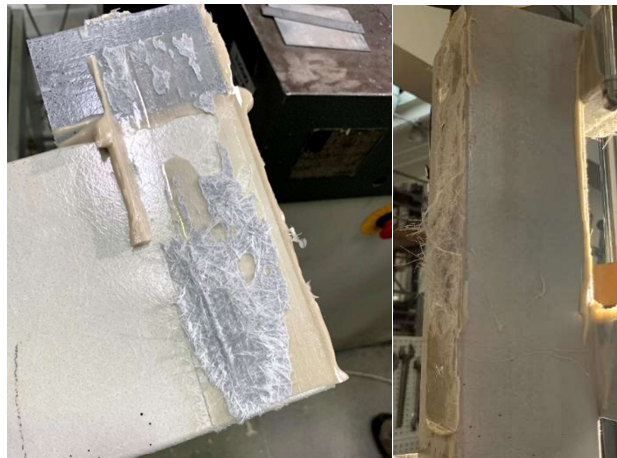
Figure 58. Mixed failure between resin and GFRP for the joint configuration of Group A.2.
