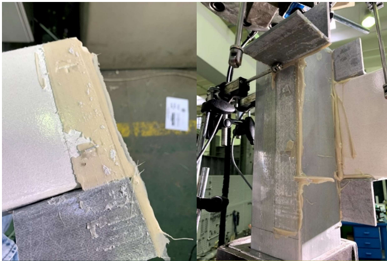
Figure 59. Cohesive failure (in the adhesive mainly) for the joint configuration of Group A.3.
