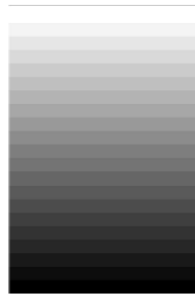
Figure 2.15. A homogenized model of a functionally graded material. [45]
