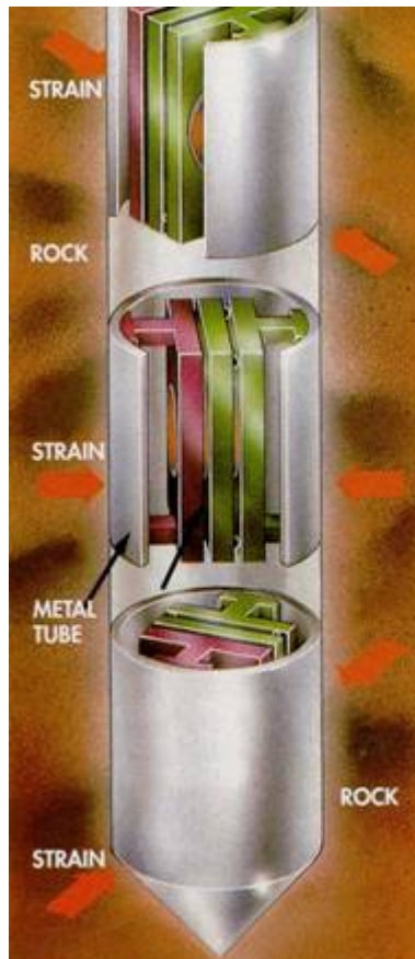
Figure 1.12: GTMS tensor strainmeter. Figure from http://www.gtsmtechnologies.com/index_files/faqs.htm .
