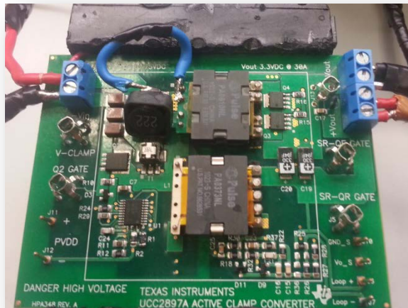
Figure 5.12 Modified UCC2897A EVM with additional inductor L_{ext}
