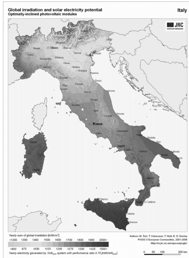
Fig. 6. 3: Global irradiation and solar electricity potential in Italy –Optimally-inclined photovoltaic modules. web site: http://www.fotovoltaicoenergiasolare.it/
