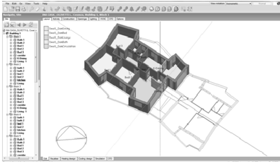
Fig. 5. 8: DesignBuilder-Ina-Olivetti, Standard Building. First floor.
