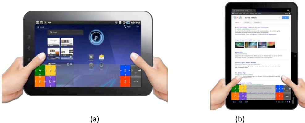
Figure 39 – tablet version of the TaS VK in the landscape modality (a) and portrait modality (b).
