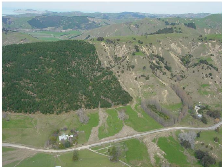
Figure 2.3 Stabilising effect of close planting of pines and riparian planting of poplars, Gisborne District, North Island, New Zealand (Crozier 2005).
