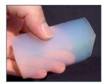
Figure 1. Silica aerogel
