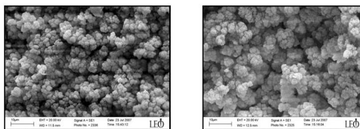
**Figure 1.8.** Comparison between monolithic polymer obtained by radiation (left) and thermally (right) polymerization.
