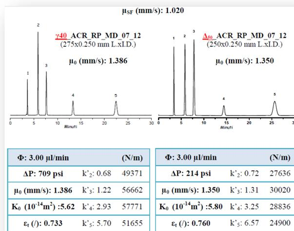
**Figure 1.9.** Comparison between monolithic columns obtained by radiation (left) and thermally (right) polymerization. 1: Uracil; 2: Benzaldehyde; 3: Nitrobenzene; 4: Ethylbenzene; 5: Butylbenzene.
