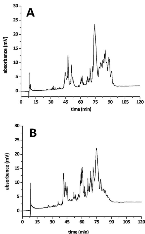
**Figure 3.9.** High-resolution (HR-Cap-LC) chromatogram of casein fraction of basal skim milk (A) and of casein fraction extracted at week IV from skim milk (B) using a 50-cm long Protein-Cap-RP-Lauryl- $\gamma$ -Monolithic column (0.250 mm I.D.). Elution: 120-min gradient from 15% to 45% of mobile phase (B); flow rate: 7  $\mu$ L/min. Tcol = 60  $^{\circ}$ C. UV detection at 214 nm. Full experimental details in Section 3.2.4.3.
