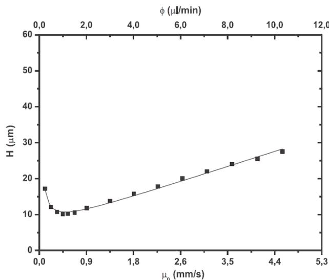
**Figure 4.3.** Experimental van Deemter for *n*-pentyl-benzene, column: Protein-Cap-RP-Lauryl- $\gamma$ -Monolithic column ( $250 \times 0.250 \text{ mm}$ ,  $L. \times I.D.$ ). Mobile phase: ACN/ $H_2O$ ; 60/40,  $v/v$ ;  $\eta$ :  $0.72 \times 10^{-3} \text{ Pa s}$  at  $25 \text{ }^\circ\text{C}$ . Column oven:  $25 \text{ }^\circ\text{C}$ ; Detection: UV at  $214 \text{ nm}$ . Injection volume:  $50 \text{ nL}$ .
