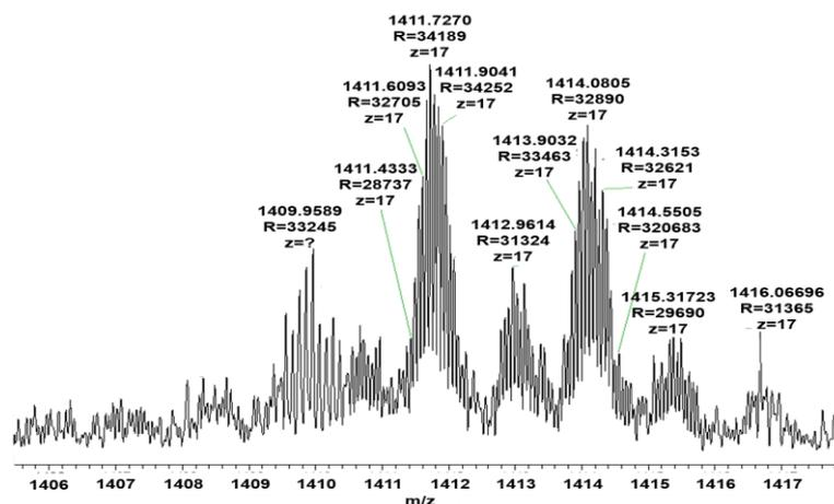
**Figure 3.4.** Expansion of mass spectrum of  $\alpha$ -CN obtained through direct infusion of a 4.0  $\mu$ M sample solution in MeCN/iso-propanol/  $H_2O/CF_3COOH$  45/45/9.9/0.1 (v/v/v/v). Instrument: LTQ Orbitrap MS ESI (+) detector.  $R = 60,000$ , mass range: 1000-2500; maximum injection time: 100ms; 1 microscan.
