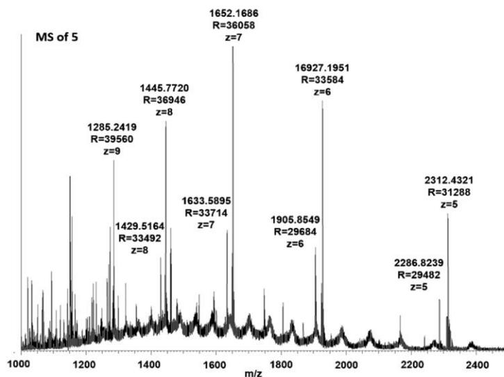
**Figure 3.13.** Mass spectrum of peak 5 in region 2 in TIC chromatogram reported in Figure 3.10. Instrument: LTQ Orbitrap MS ESI (+) detector.  $R = 60,000$ , mass range: 1000–3000; maximum injection time: 100 ms for 1 microscan.
