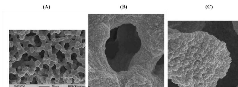
**Figure 1.2.** SEM-image of the porous structure of a typical monolithic silica column (A), enlarged view of the entrance to a macropore or throughpore (B) and mesoporous structure of the skeleton (C).
