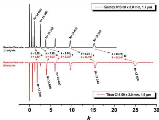
**Figure 4.12.** Comparison of isocratic elution on the Kinetex<sup>TM</sup> C18 50 × 3.0 mm, 1.7  $\mu\text{m}$  (black line), Titan<sup>TM</sup> C18 50 × 3.0 mm, 1.9  $\mu\text{m}$  (red dotted line). Column oven: 35 °C; Detection: UV at 214 nm, Sampling rate: 80 points/s; resolution: 4.8 nm; no filter. Injection volume: 0.5  $\mu\text{L}$ . Sample: small molecule mixture. Results are expressed as retention factors ( $k$ ) and theoretical plates per column ( $N$ ).
