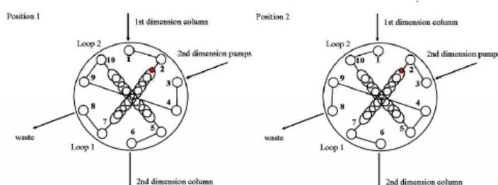
**Figure 1.15.** 10-port two-position switching valve.
