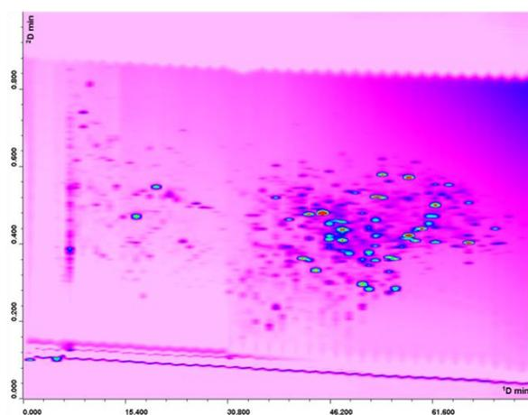
**Figure 4.15.** 2D LC  $\times$  UHPLC plot of peptides  $< 3,000$  Da fraction after four week from expiration date.  $^1\text{D}$  column Discovery<sup>®</sup> 150  $\times$  1.0 mm, 5  $\mu\text{m}$ ; flow rate 20  $\mu\text{L}/\text{min}$ ; column oven: 25  $^\circ\text{C}$ ; injection volume 2  $\mu\text{L}$ .  $^2\text{D}$  column Kinetex<sup>TM</sup> C18 50  $\times$  3.0 mm, 1.7  $\mu\text{m}$ ; flow rate 2.5 mL/min. Modulation time 60 sec; column oven: 60  $^\circ\text{C}$ .
