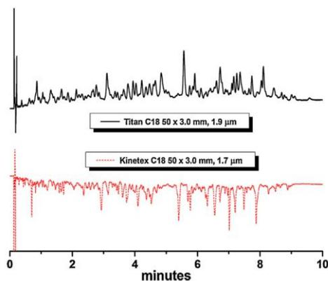
**Figure 4.13.** Comparison of a fast gradient elution on the Kinetex<sup>TM</sup> C18 50 × 3.0 mm, 1.7  $\mu\text{m}$  (red dotted line), Titan<sup>TM</sup> C18 50 × 3.0 mm, 1.9  $\mu\text{m}$  (black line). Instrument: Waters UPLC; Detector: PDA; Cell: 500 nL; UV at 214 nm; Tcol: 40 °C; Vinj: 6.0  $\mu\text{L}$ ; Mobile phase: (A) H<sub>2</sub>O/ACN 95/5 v/v + 0.1% v/v TFA; (B) ACN/H<sub>2</sub>O 95/5 v/v + 0.1% v/v TFA; Flow rate: 1.5 mL/min. Sample: peptides < 3,000 Da fraction.
