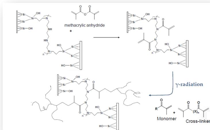
**Figure 1.6.** Reaction scheme of derivatization “Grafting-on-to”.
