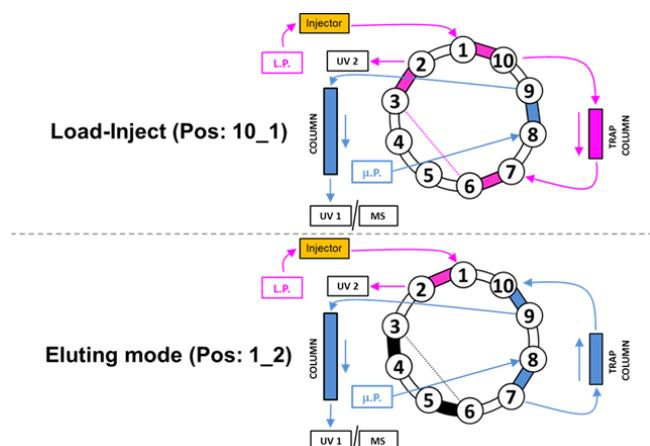
**Figure 3.1.** Sketch of 10-valve port used for load-trapping purposes.
