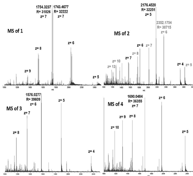
**Figure 3.11.** Mass spectra of peaks 1–4 in region 1 in TIC chromatogram reported in Figure 3.10. Instrument: LTQ Orbitrap MS ESI (+) detector.  $R = 60,000$ , mass range: 1000–3000; maximum injection time: 100 ms for 1 microscan.
