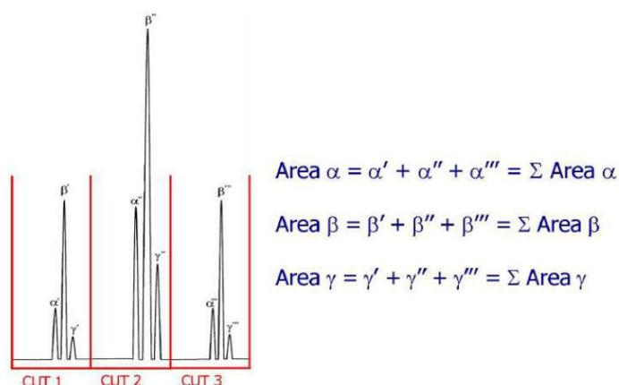
**Figure 1.12.** *Quantitative procedure in LC × LC.*
