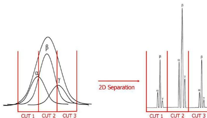
**Figure 1.11.** Effects of modulation on 3 co-eluting peaks.
