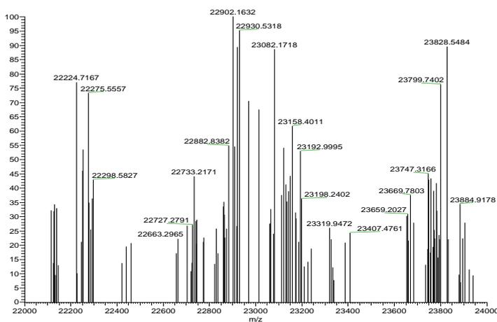
**Figure 3.14.** Range of exact molecular masses of  $\alpha_{S1}$ -CN. Monoisotopic exact molecular masses were obtained by deconvolution of high resolution mass spectrum 5 in Figure 3.13. using Xtract software.
