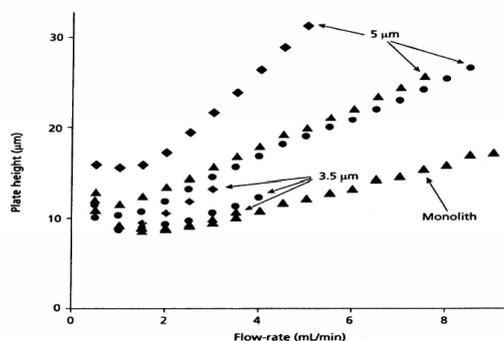
**Figure 1.3.** Comparison of the efficiency of particle-packed and monolithic columns.
