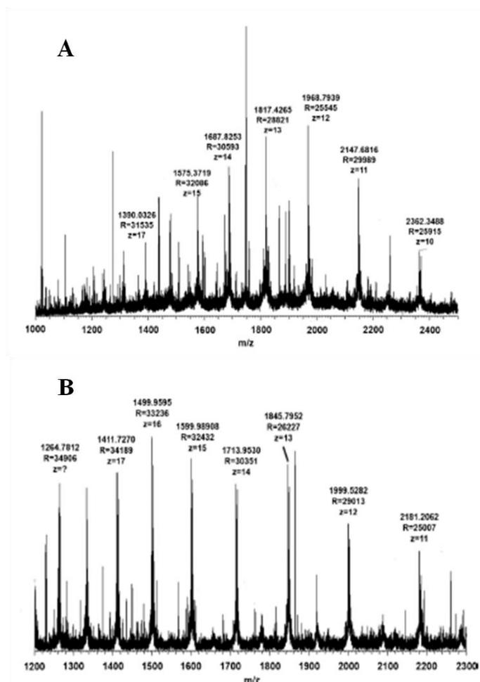
**Figure 3.3.** Mass spectra of  $\alpha_s$ -CN (A) and  $\beta$ -CN (B) obtained through direct infusion of a 4.0  $\mu$ M sample solution in MeCN/iso-propanol/ $H_2O$ / $CF_3COOH$  45/45/9.9/0.1 (v/v/v/v). Instrument: LTQ Orbitrap MS ESI (+) detector.  $R = 60,000$ , mass range: 1000–2500; maximum injection time: 100 ms; 1 microscan.
