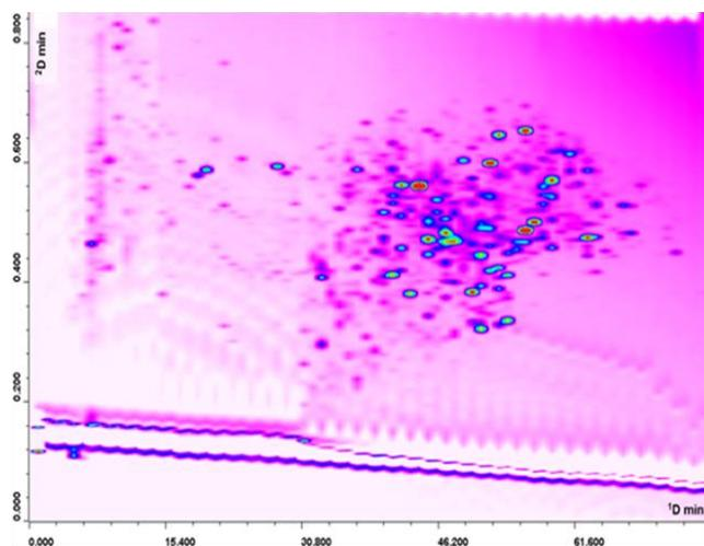
**Figure 4.14.** 2D LC  $\times$  UHPLC plot of peptides  $< 3,000$  Da fraction after four week from expiration date.  $^1\text{D}$  column Discovery<sup>®</sup> 150  $\times$  1.0 mm, 5  $\mu\text{m}$ , flow rate 20  $\mu\text{L}/\text{min}$ ; column oven: 25  $^\circ\text{C}$ , injection volume 2  $\mu\text{L}$ .  $^2\text{D}$  column Titan<sup>TM</sup> C18 50  $\times$  3.0 mm, 1.9  $\mu\text{m}$ .; flow rate 2.5 mL/min. Modulation time 60 sec; column oven: 60  $^\circ\text{C}$ .
