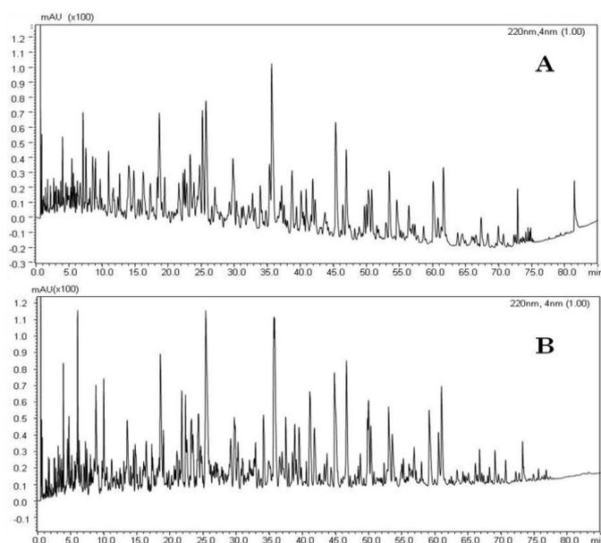
**Figure 4.19.** Chromatograms of high efficiency monodimensional comparative analysis of the peptides belonging to < 3,000 Da fraction. Titan<sup>TM</sup> C18 2  $\times$  100  $\times$  2.1 mm, 1.9  $\mu\text{m}$ ,  $n_c$ : 454 (A); Kinetex<sup>TM</sup> C18 100 + 50  $\times$  2.1 mm, 1.7  $\mu\text{m}$ ,  $n_c$ : 490 (B).
