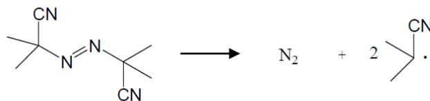
**Figure 1.7.** Decomposition reaction of azobisisobutyronitrile.
