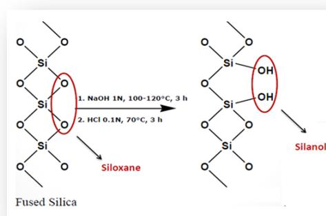
**Figure 1.4.** Activation of inner wall surface of fused silica capillary.
