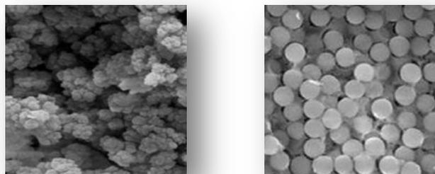
**Figure 1.1.** Comparison between monolithic (left) and packed stationary phases (right).
