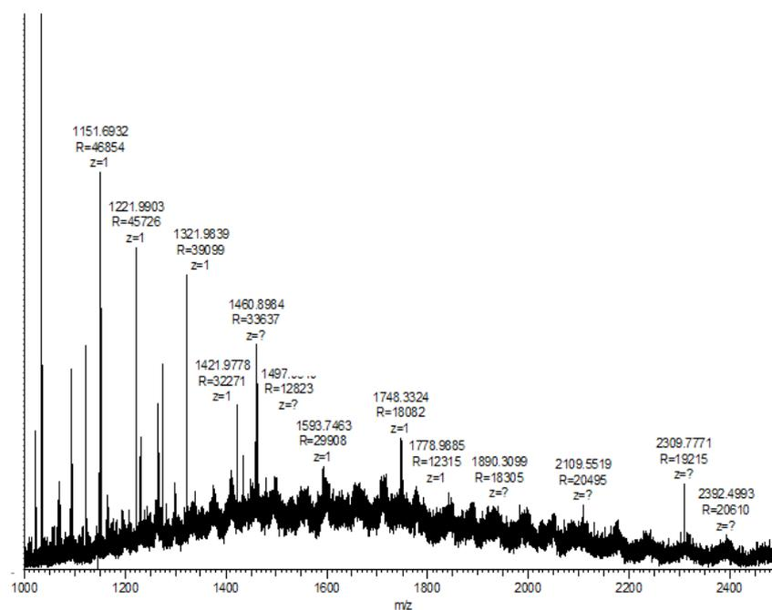
**Figure 3.12.** Mass spectrum of peak 6 of TIC chromatogram in Figure 3.10. (see text). Instrument: LTQ Orbitrap MS ESI (+) detector. R = 60,000, mass range: 1000-3000; maximum injection time: 100 ms for 1 microscan.
