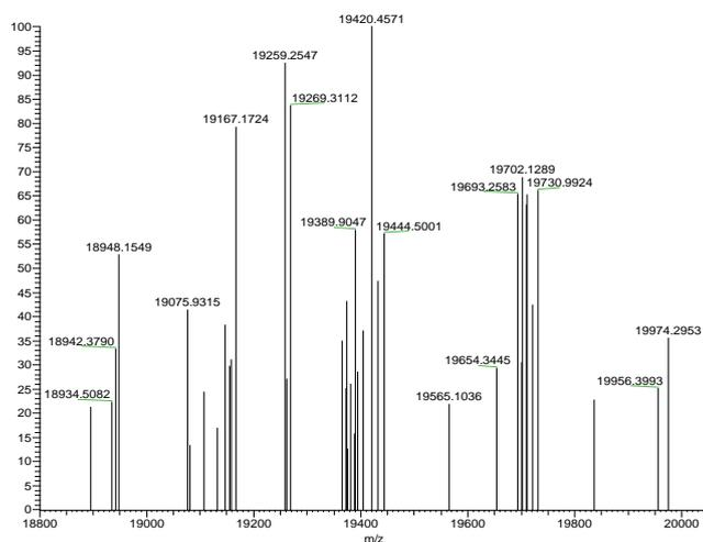
**Figure 3.16.** Range of exact molecular masses of  $\kappa$ -CN. Monoisotopic exact molecular masses were obtained by deconvolution of high resolution mass spectrum 5 in Figure 3.13. (see text) using Xtract software.
