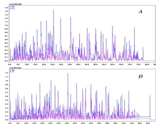
**Figure 4.20.** Total ion chromatograms of high efficiency monodimensional comparative analysis of the peptides < 3,000 Da fraction. Columns top: Titan<sup>TM</sup> C18 2  $\times$  100  $\times$  2.1 mm, 1.9  $\mu\text{m}$ ; bottom: Kinetex<sup>TM</sup> C18 100 + 50  $\times$  2.1 mm, 1.7  $\mu\text{m}$ .
