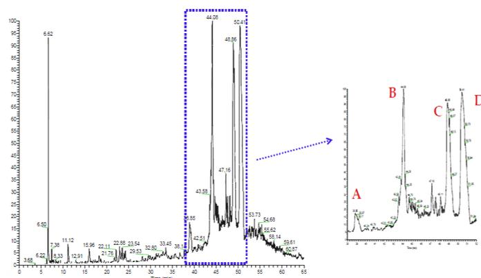
**Figure 4.5.** Total ion current of whey fraction using a 250 cm long protein-Cap-RP-Lauryl- $\gamma$ -Monolithic column (0.250 mm I.D.). Elution: 70-min gradient from 15% to 45% of mobile phase (B); flow rate: 10  $\mu\text{L}/\text{min}$ . Tcol = 60  $^{\circ}\text{C}$ . Exactive Orbitrap MS-ESI (+) detector. R = 10,000, mass range: 500-4000 amu. Full experimental details in Section 4.2.6.2.
