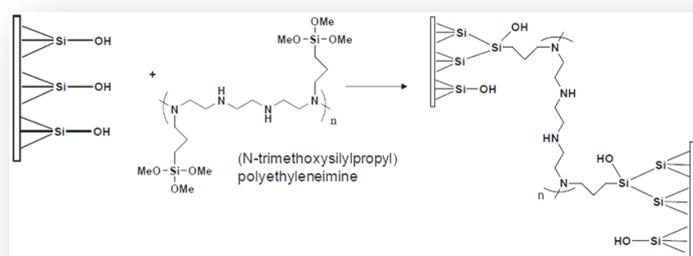
**Figure 1.5.** Reaction scheme of silanating “Tentacle type”.
