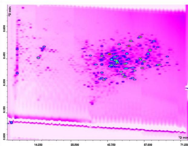
**Figure 4.17.** 2D LC  $\times$  UHPLC plot of peptides  $< 3,000$  Da fraction after four weeks from expiration date. 1D column Discovery® 150  $\times$  1.0 mm,  $\mu\text{m}$ ; flow rate 20  $\mu\text{L}/\text{min}$ ; column oven: 25  $^{\circ}\text{C}$ ; injection volume 2  $\mu\text{L}$ . 2D column Kinetex<sup>TM</sup> C18 50  $\times$  3.0 mm, 1.7  $\mu\text{m}$ ; flow rate 2.5 mL/min. Modulation time 45 s; column oven: 60  $^{\circ}\text{C}$ .
