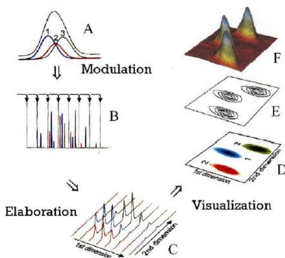
**Figure 1.14.** Data elaboration in comprehensive two-dimensional HPLC: (A) 1D non-modulated peak; (B) modulated 2D peaks; (C) fractions of modulated peaks, analyzed in 2 dimensions; (D) bidimensional data visualization (color); (E) bidimensional data visualization (grayscale); (F) three-dimensional visualization.
