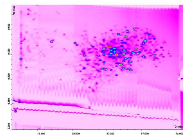
**Figure 4.16.** 2D LC  $\times$  UHPLC plot of peptides  $< 3,000$  Da fraction after four weeks from expiration date. 1D column Discovery® 150  $\times$  1.0 mm, 5  $\mu\text{m}$ , flow rate 20  $\mu\text{L}/\text{min}$ ; column oven: 25  $^{\circ}\text{C}$ , injection volume 2  $\mu\text{L}$ . 2D column Titan<sup>TM</sup> C18 50  $\times$  3.0 mm, 1.9  $\mu\text{m}$ ; flow rate 2.5 mL/min. 2D Modulation time 45 s; column oven: 60  $^{\circ}\text{C}$ .
