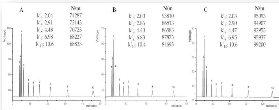
**Figure 4.2.** Chromatographic characterization and efficiency test of Protein-Cap-RP-Lauryl- $\gamma$ -Monolithic column (250  $\times$  0.250 mm L.  $\times$  I.D.). (A):  $\Phi$ : 3.00  $\mu\text{L}/\text{min}$ ,  $\Delta P_c$ : 817 psi; (B)  $\Phi$ : 2.00  $\mu\text{L}/\text{min}$ ,  $\Delta P_c$ : 523 psi;  $\Phi$ : 1.00  $\mu\text{L}/\text{min}$ ,  $\Delta P_c$ : 287 psi.
