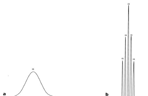
**Figure 1.10.** Non-modulated peak  $\alpha$  (a) and peak  $\alpha$  modulated 5 times (b).
