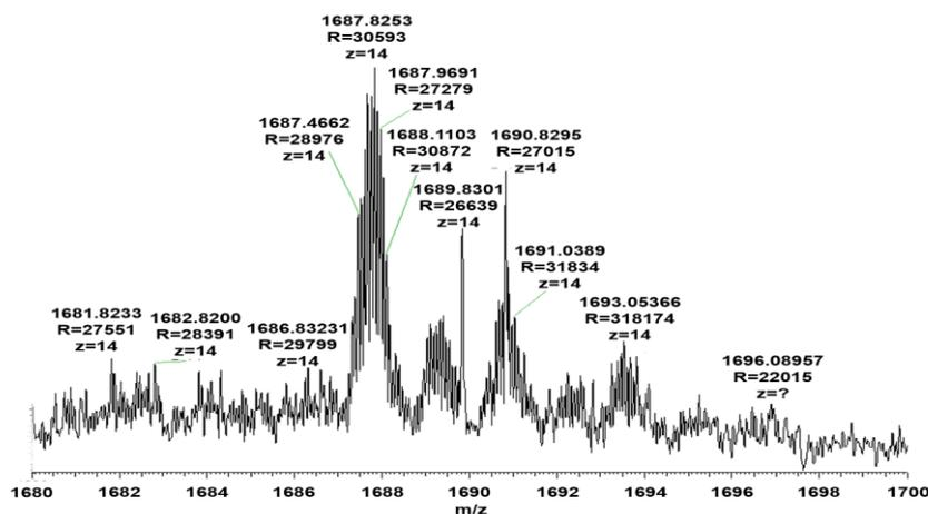
**Figure 3.5.** Expansion of mass spectrum of  $\beta$ -CN obtained through direct infusion of a 4.0  $\mu$ M sample solution in MeCN/iso-propanol/  $H_2O/CF_3COOH$  45/45/9.9/0.1 (v/v/v/v). Instrument: LTQ Orbitrap MS ESI (+) detector.  $R = 60,000$ , mass range: 1000-2500; maximum injection time: 100ms; 1 microscan.
