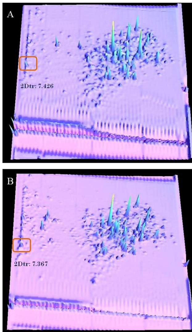
**Figure 4.18.** Three dimensional projection of 2D LC  $\times$  UHPLC plot of peptides  $< 3,000$  Da fraction obtained using in second dimension a (A) Titan™ C18 and (B) Kinetex™ C18 columns, respectively, with a modulation time of 45 s. The LC  $\times$  LC data were visualized and elaborated in three dimensions using Chromsquare® ver. 1.5.01 software.
