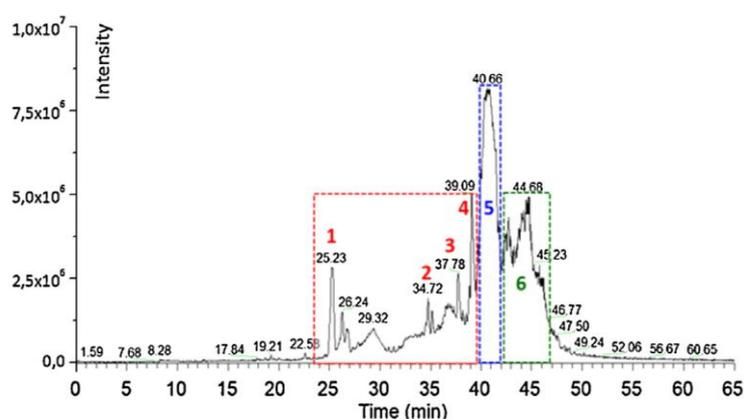
**Figure 3.10.** Total ion current chromatogram (Cap-LC–HRMS analysis) of casein fraction extracted at week IV from skim milk (B) using a 50-cm long protein-Cap-RP-lauryl- $\gamma$ -monolithic column (0.250 mm I.D.). Elution: 60-min gradient from 15% to 45% of mobile phase (B); flow rate: 7  $\mu$ L/min. Tcol = 60 °C. UV detection at 214 nm. LTQ Orbitrap MS ESI (+) detector. R = 60,000, mass range: 1000–3000 amu. Full experimental details in Section 3.2.6.
