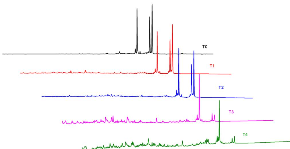
**Figure 4.10.** *Chromatographic profile of whey fraction extracted from semi-skimmed milk at weeks I-IV from expiry date. Column: Protein-Cap-RP-Lauryl- $\gamma$ -Monolithic (25 cm  $\times$  0.250 mm, L.  $\times$  I.D.). Elution: from 10% to 35% of mobile phase B with a 70-min gradient time; flow rate: 10  $\mu\text{L}/\text{min}$ . Tcol = 60  $^{\circ}\text{C}$ . UV detection at 214 nm. See Section 4.2.6.1. for full experimental details.*
