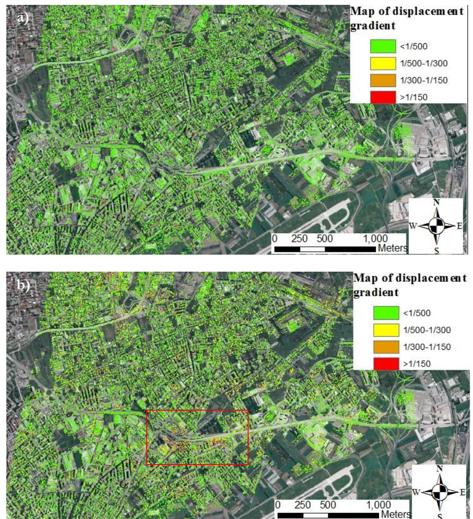
Figure 6.27. Map of displacement gradients in the surrounding area of Naples Airport with reference to: a) period 2010-2011; b) period 2011-2021.
