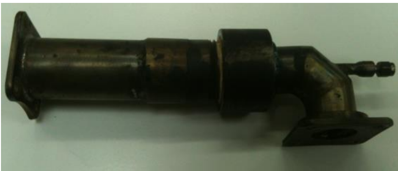
Figure 2.7: Image of a CPOx reactor used in a \mu CHP application [38]
