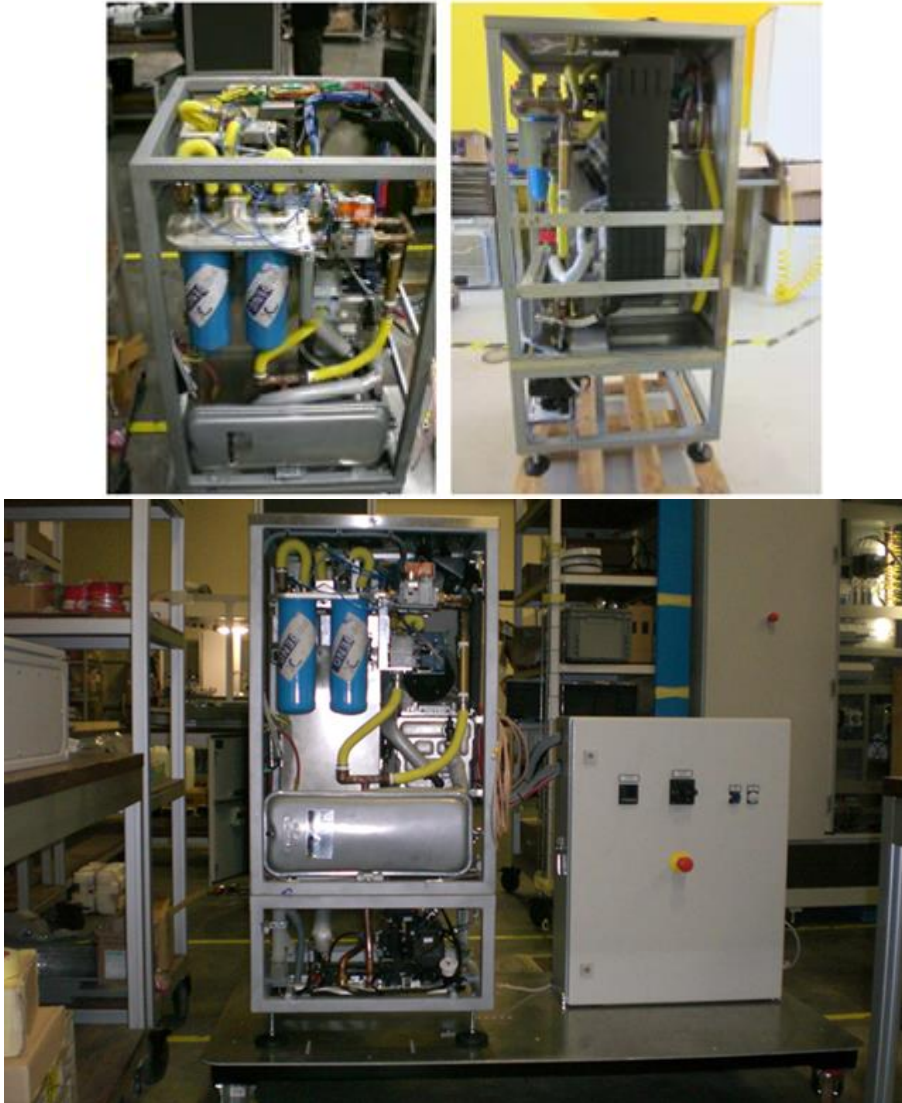
Figure 3.13 – 1 kW \mu CHP realized by Ariston Thermo [103]
