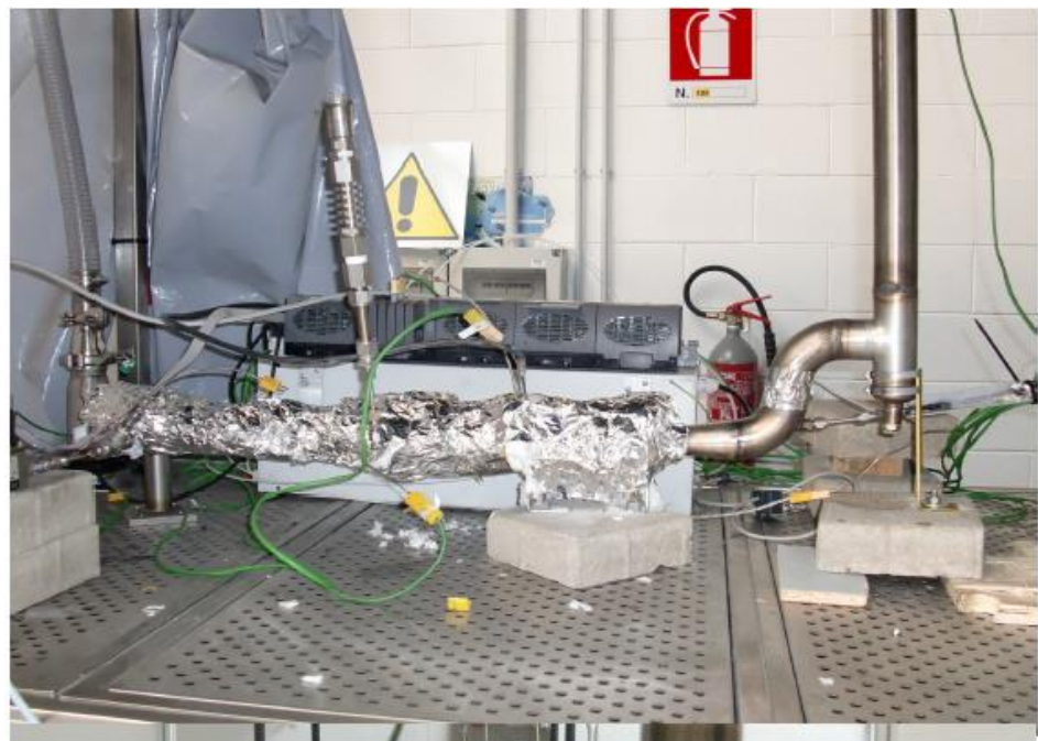
Figure 3.9 – CPOx reactor test bench setup (Hysylab) [102]
