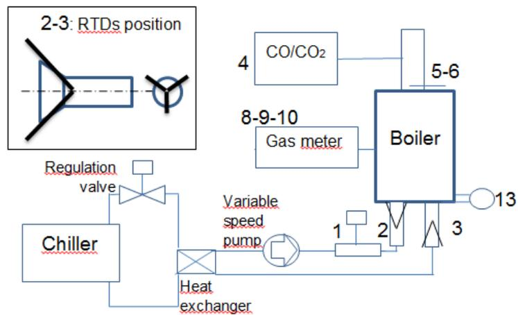
Figure 2. Boiler efficiency measurement apparatus, instruments label refers to Table 2.
