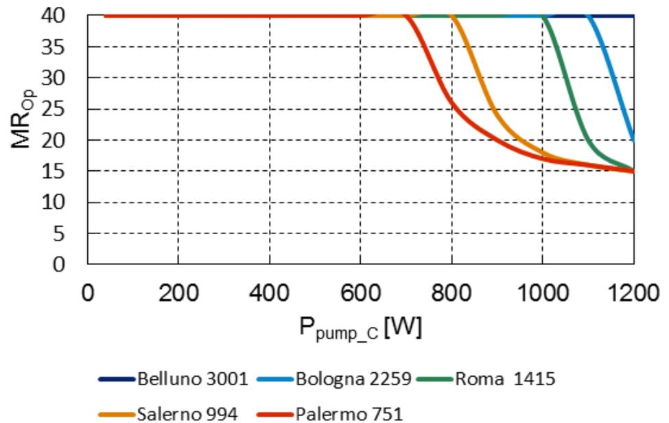
**Figure 33. Optimal maximum modulation ratio as a function of electrical power for different Italian cities.**
