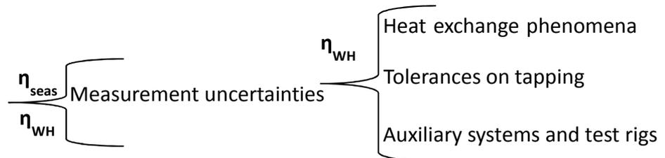
**Figure 11. Laboratory and production effects on water heating and space heating efficiencies uncertainty**
