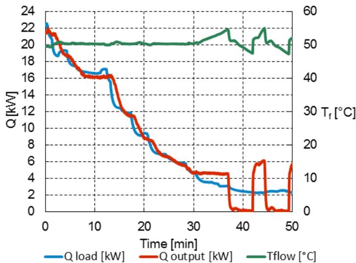
**Figure 1. Example of boiler cycling to satisfy a load lower than minimum heat output.**
