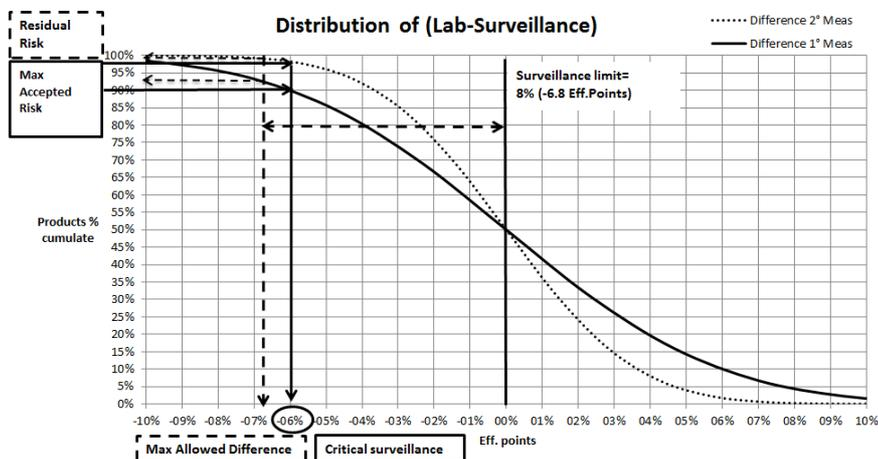
Figure 13. Surveillance tolerance on water efficiency analysis on storage boiler assuming an acceptable risk of non-conformity.
