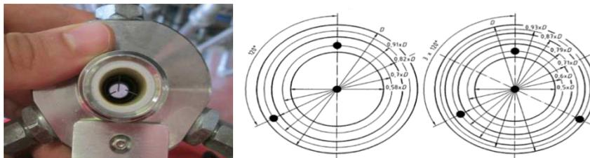
Figure 5. Thermocouples positioning with surface methods.
