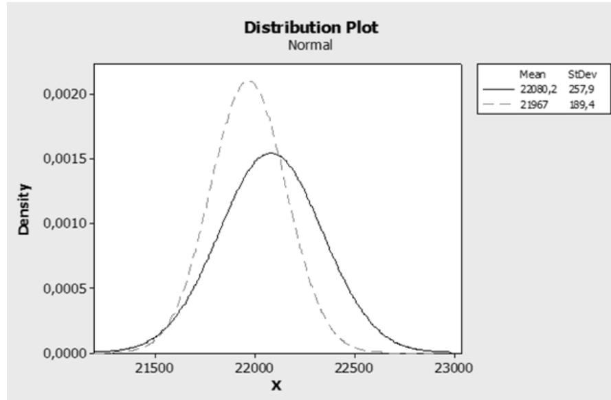
Figure 9. Comparison of the statistical distribution of heat input and global heat output measurements
