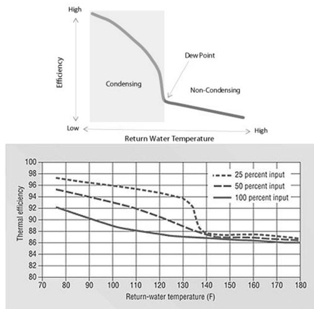
**Figure 24. Boiler efficiency increase due to condensation as a function of water return temperature and heat input**
