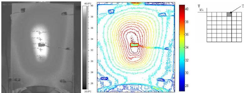
**Figure 18. Boiler frontal thermal camera measurement during burning phase and correspondent Matlab elaboration**
