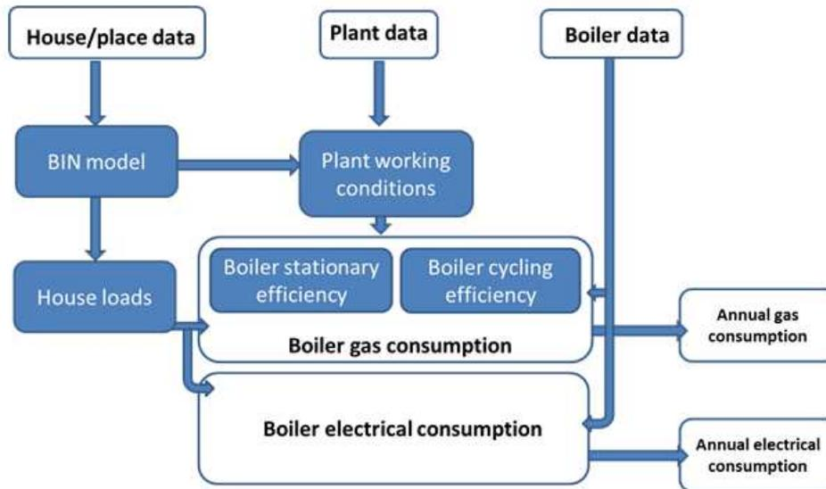
**Figure 25. Model overview: on the top model inputs and on the right the model output. Model is composed by different sub-models: bins model, house loads calculation, plant model and boiler consumption submodels**
