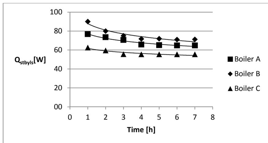
**Figure 17. Boiler standby losses results for three differently insulated boilers**
