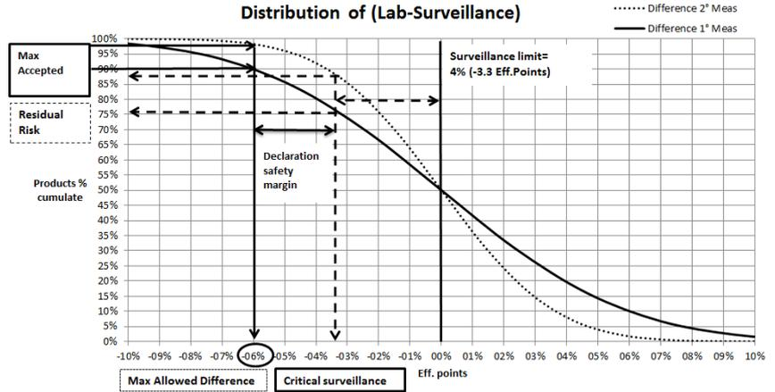
**Figure 14. Surveillance tolerance on water efficiency analysis on storage water heater assuming an acceptable risk of non-conformity.**
