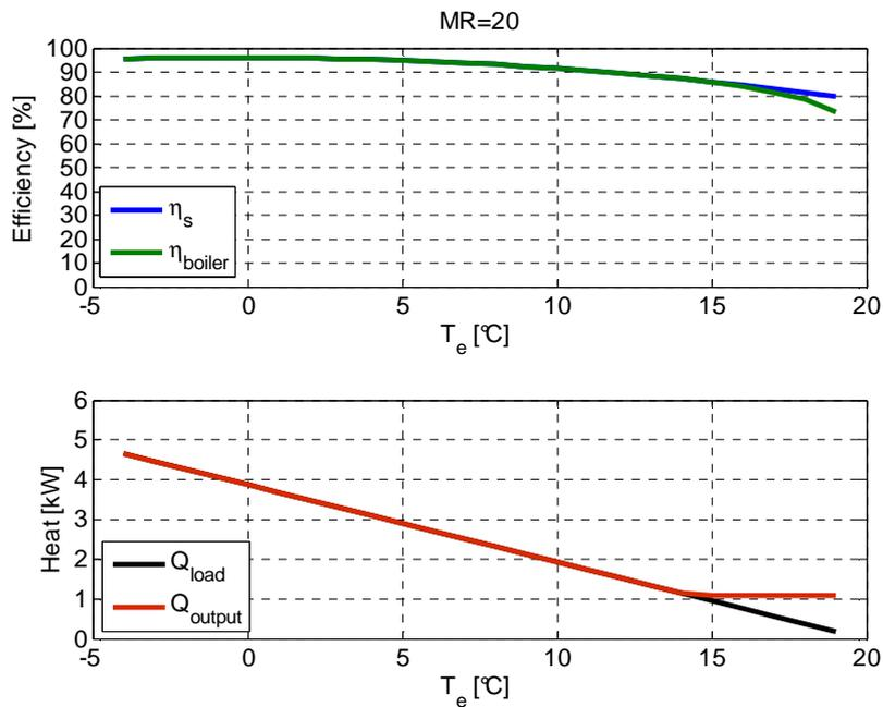
**Figure 31. For a boiler with maximum modulation ratio equal to 20: in top figure the efficiency degradation due to cycling losses, in the second one, boiler heat output and loads as a function of external temperature**
