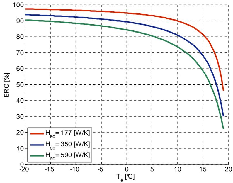
**Figure 28. Boiler efficiency reduction from stationary conditions due to cycling losses (ERC) as a function of the external temperature for a fixed boiler and different building specific losses.**
