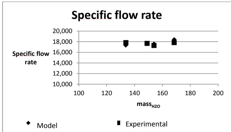
Figure 21. Experimental and modeled specific flow rate is reported for different tapped water quantities for a 22kW and 40 liters storage boiler. Model well approximates SR experimental results.
