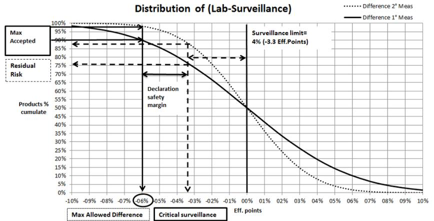
**Figure 14. Surveillance tolerance on water efficiency analysis on storage water heater assuming an acceptable risk of non-conformity.**
