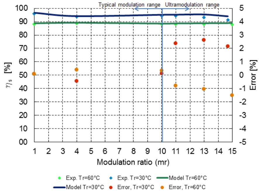
**Figure 27. Boiler efficiency experimental, modeled and relative error. Boiler delta water temperature is fixed and equal to 20°C. Data are divided into modulation and ultra-modulation range.**
