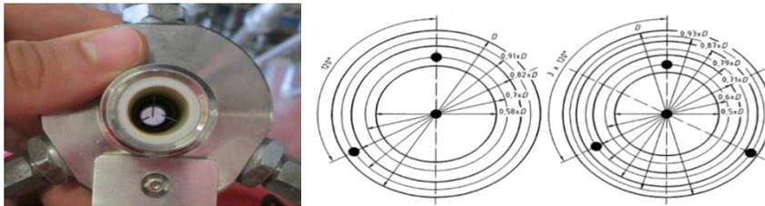
Figure 5. Thermocouples positioning with surface methods.
