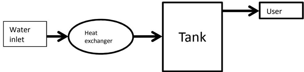
Figure 19. Boiler burner/tank logic scheme for sanitary draw-off
