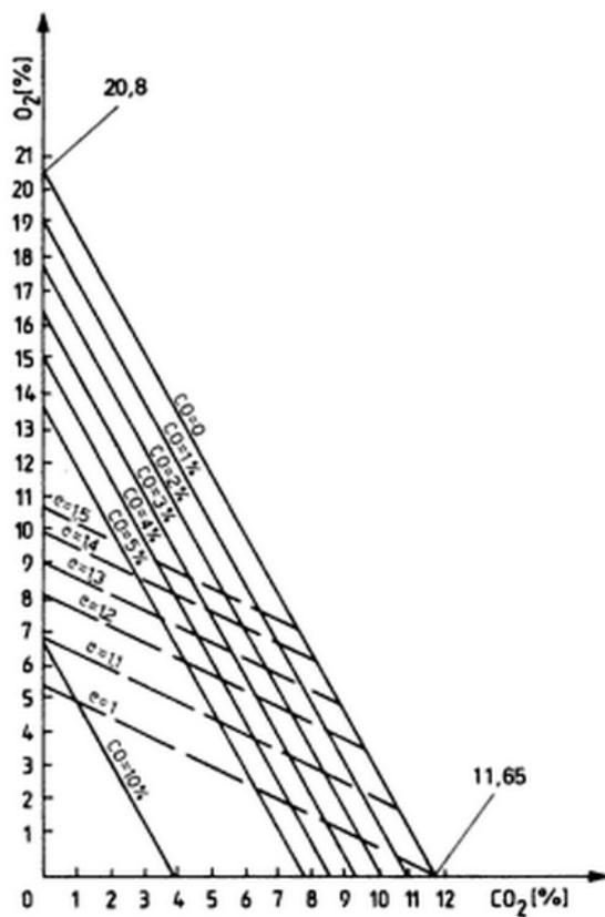
Figure 23. Ostwald triangle for methane – The triangle correlate air excess “e” with  $CO$ ,  $CO_2$  and  $O_2$  concentrations determining the combustion conditions.
