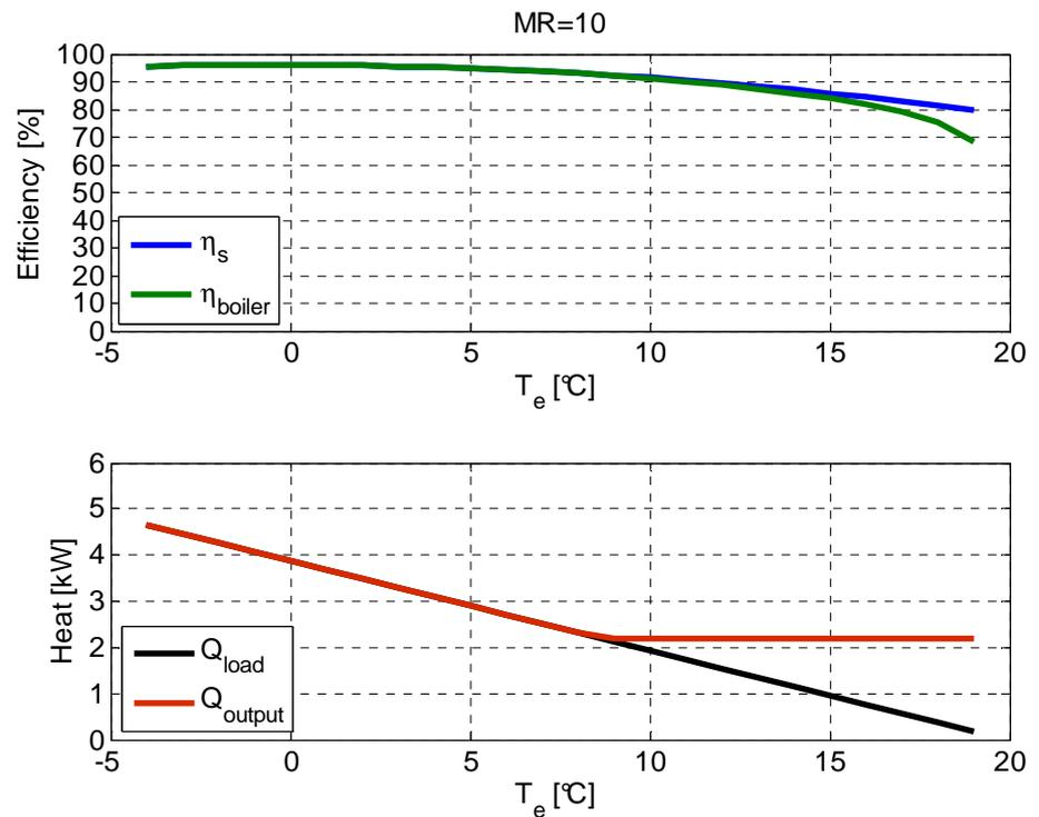
**Figure 30. For a boiler with maximum modulation ratio equal to 10: in top figure the efficiency degradation due to cycling losses, in the second one, boiler heat output and loads as a function of external temperature.**
