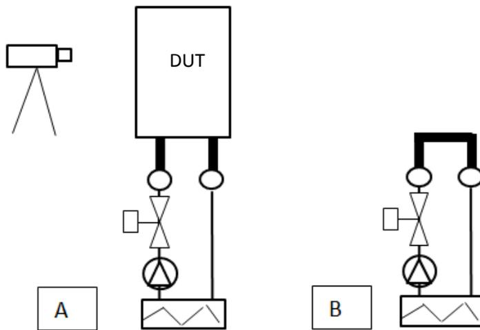
**Figure 16. B represents the test bench loss characterization while A the DUT measurement test.**
