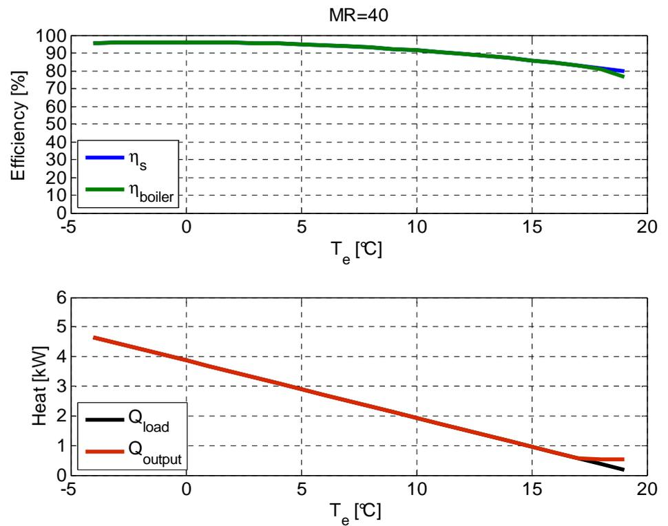
**Figure 32.** For a boiler with maximum modulation ratio equal to 40: in top figure the efficiency degradation due to cycling losses, in the second one, boiler heat output and loads as a function of external temperature.
