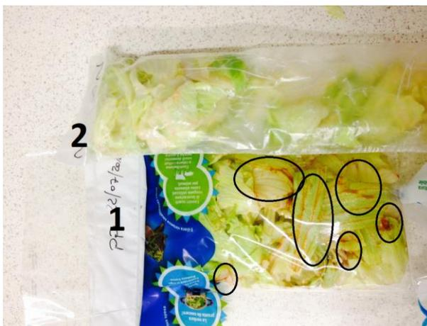
**Fig 2.4.12** Salad packaging in BOPP film and in PP-sPS-PP crystallized film. With symbol O maceration are indicated
