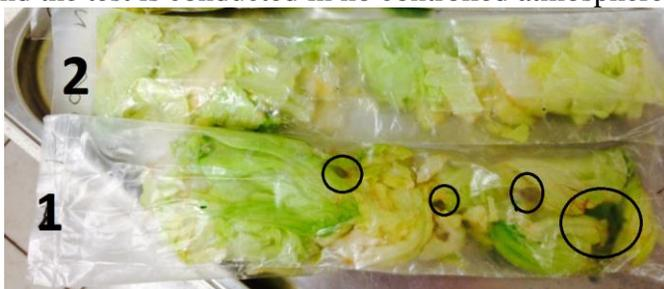
**Fig 2.4.11** Salad iceberg packaging in PP-sPS-PP films: 1) Amorphous 2) crystallized with eco-friendly solvent 3) crystallized with non-eco-friendly solvent. With symbol O maceration is indicated.
