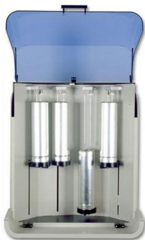
Figure 22: Nova 3000e, Quantachrome, USA- Brunauer Emmett Teller measurements.
