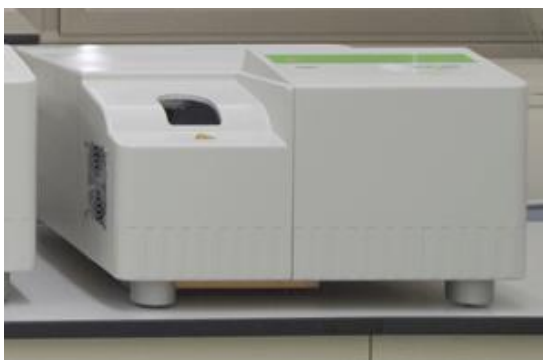
Figure 17: DSC 822e Mettler Toledo apparatus.
