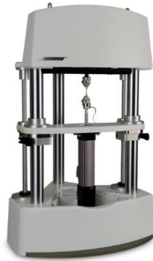
Figure 20: Tensile stress tester Electroforce 3200 Bose, Eden Praire.
