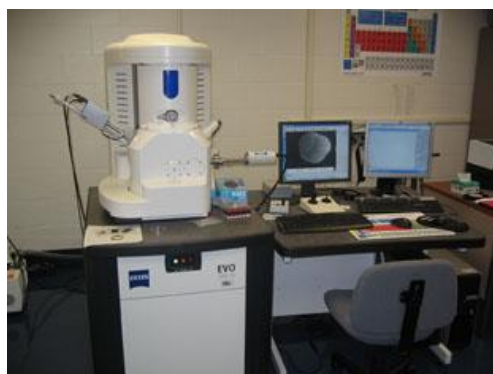
Figure 18: Scanning Electron microscope Evo Zeiss MA 10.
