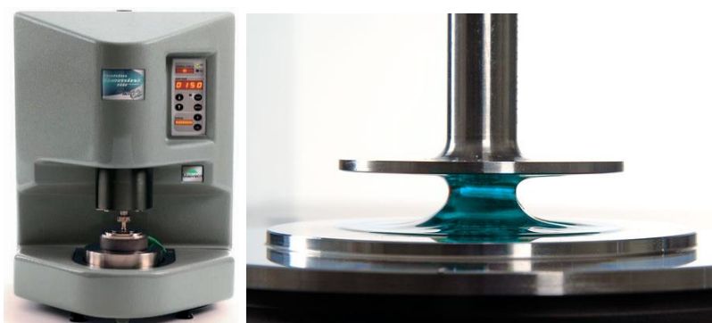
Figure 23 Image of Bohlin CS rheometer instrument
