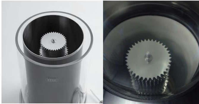
Figure 9: The Nano spray drier electrostatic particle collector: On the left clean and on the right with particles attached.
