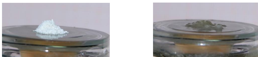
Figure 46: Gelification of a GAP powder in 15 minutes when in contact with simulated wound fluid.
