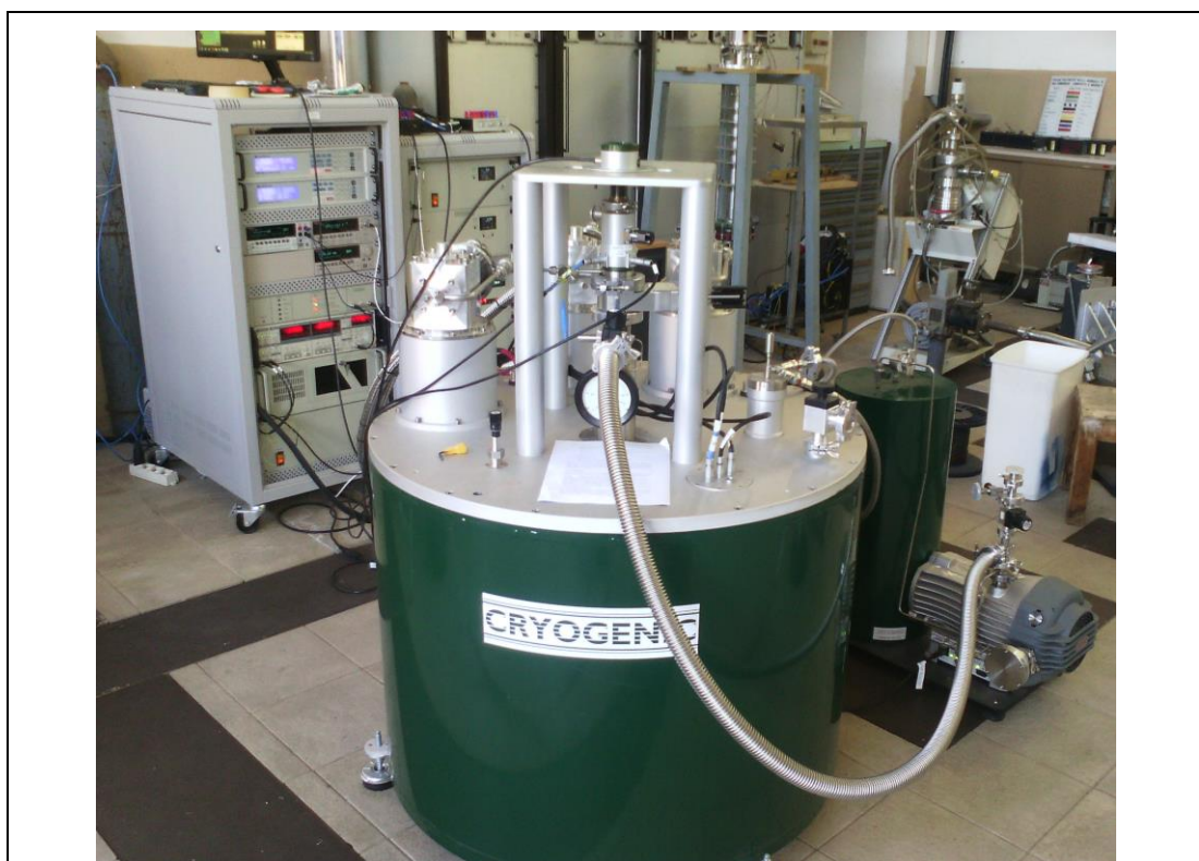
Figure 11: Cryogenic Ltd. cryogen free cryostat for transport and magnetic measurements up to 18 T at Superconductivity Laboratories, ENEA C.R. Frascati.
