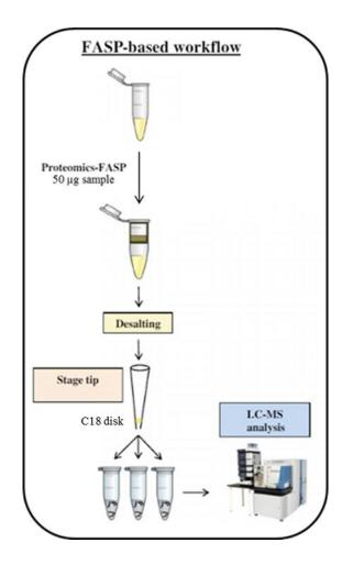
**Figure 3.5.** Proteomic workflow. FASP method is followed by StageTip desalting to prepare samples for the proteome data set.
