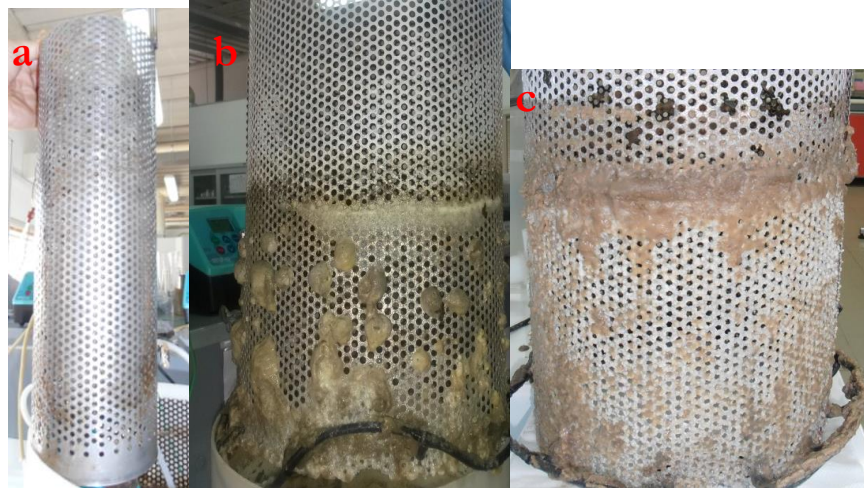
Figure 6.8 Pictures of the cathode at the end of the second (eMBR-1) and third (eMBR-3) run (a), anode at the end of the second run (eMBR-1) (b) and of the third run (eMBR-3) (c).
