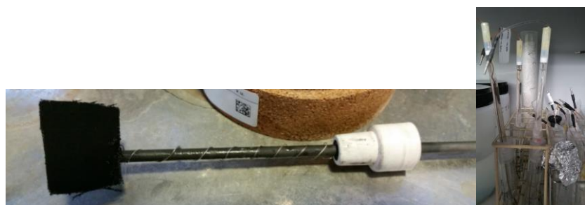
Figure 5.9 Working and counter electrodes with carbon clothes and graphite bar on the left and Ag/AgCl reference electrode on the right.
