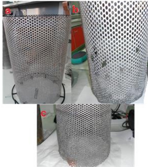
Figure 6.5 Aluminium anode at the start of the experimental runs (a), at the end of the second run (eMBR-1) and of the third run (eMBR-3).
