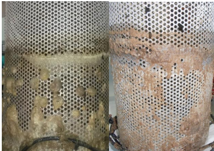
Figure 6.4 Biomass found attached on the anode electrode at the end of the second run (eMBR-1) and at the end of the third run (eMBR-3).
