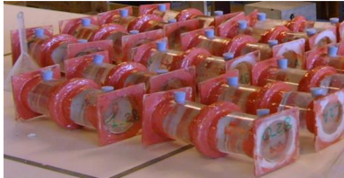
Figure II.4 Test setup for Chloride diffusion test
