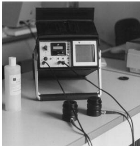
Figure II.5 Test setup and equipment for Dynamic Modulus of Elasticity test.
