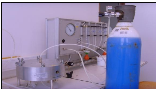
Figure II.2 Test cell and apparatus for Oxygen Permeability test
