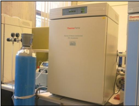
Figure II.3 Test sample and equipment for carbonation resistance test
