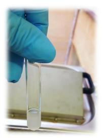
Figure 77 The dry lipid film formed at the bottom of the vial was suspended in sucrose buffer
