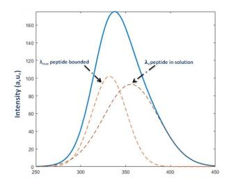
Figure 80 An example of how a deconvolution analysis works
