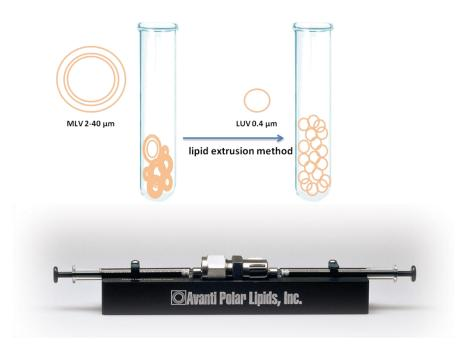
Figure 78 Avanti polar lipids extruder used to generate LUV of 0.4  $\mu M$  from MLV
