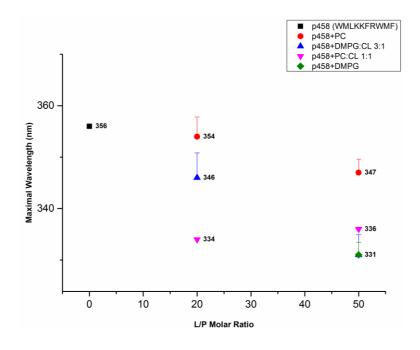
Figure 82 Fluorescence emission of the peptide p458 when it interacts with PC, DMPG, DMPG:CL 3:1 and PC: CL 1:1 vescicles. The maximal wavelength of Trp fluorescence is plotted as a function of L/P molar ratio.
