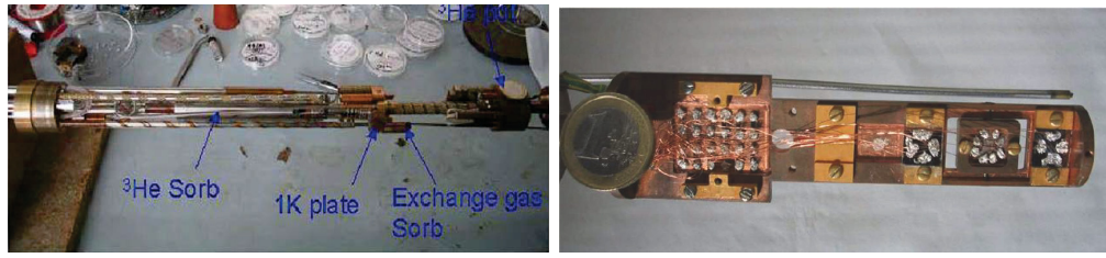
Figure 2.33: (left) Picture of the inner IVC chamber. (right) Picture of the sample holder.
