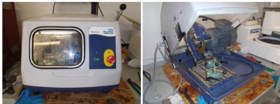
Figure 4.8 – Delta AbrasiMet bench-top cutter
