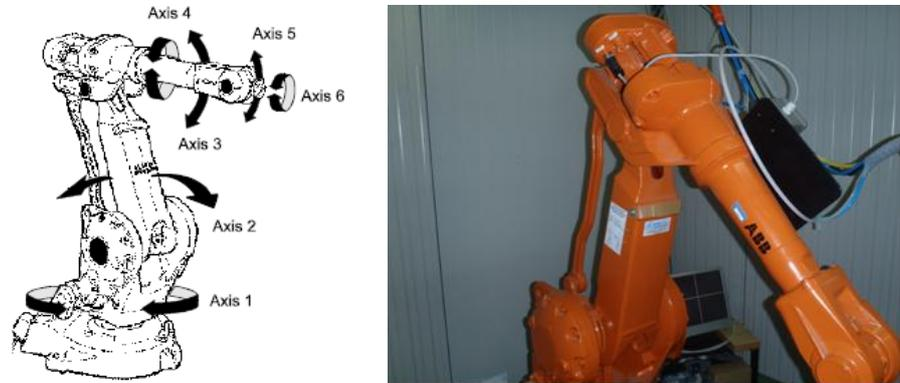
Figure 4.5 – Robot ABB IRB 2400
