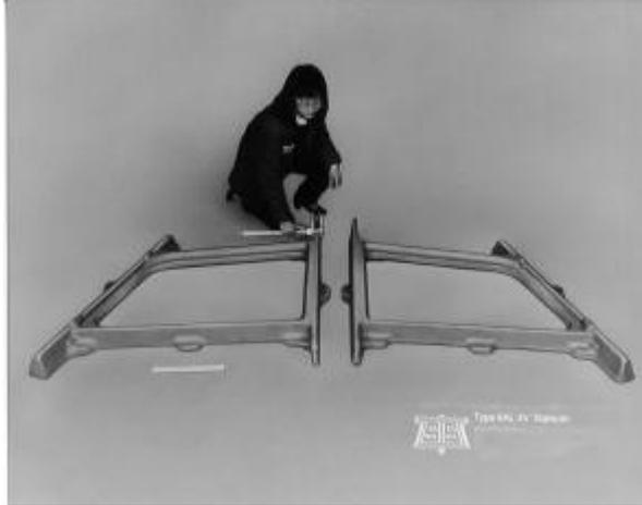
**Figure 2.12 – Window frames of Ti-6Al-4V for the cockpit of a commercial aircraft**
