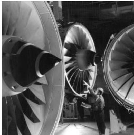
**Figure 2.15 – Front fans of commercial Rolls- Royce Trent engines made of Ti-6Al-4V**
