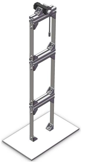
The length of the structural elements are equal respectively to  $L_1 = 23 \cdot 10^{-2} [m]$ ,  $L_2 = 28 \cdot 10^{-2} [m]$  and  $L_3 = 23 \cdot 10^{-2} [m]$  whereas the half-length of the pendulum is equal to  $L_4 = 8.25 \cdot 10^{-2} [m]$ . The dimensions of the cross sections relative to the structural elements are  $b_1 = b_2 = b_3 = 3.5 \cdot 10^{-2} [m]$
