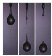
Figure 7. Example of "satellite" particles formation.
