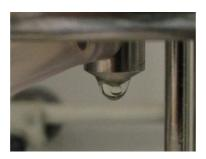
Figure 8. Example of core-shell particle formation by co-axial prilling.
