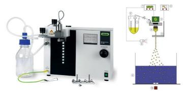
Figure 10. Büchi encapsulator B-390 apparatus
