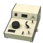
Figure 18. Quanta-Chrome MPY-2 Helium Micropycnometer.
