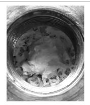
Figure III.17 Photographs of foaming materials in the saturator.
