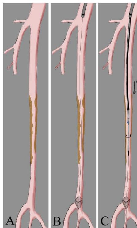
**Fig. 1.** Illustration of the Turbohawk™ device. **A.** Multiple preocclusive SFA stenosis. **B.** Deployment of distal protection device. **C.** Plaque excision with Turbohawk™ (description of the technique in the text).
