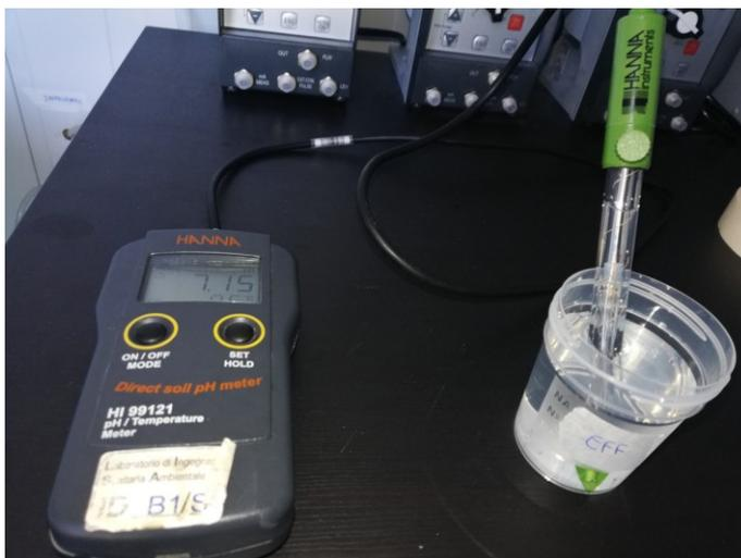
Figura 5.49 Sonda multiparametrica Hanna Instruments HI99121
