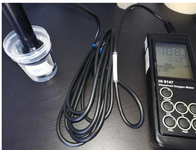
**Figura 5.48 Sonda Hanna Instruments HI9147**
