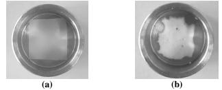
*Figure V.32 Photographs of (a) unprocessed PCL film; (b) foamed PCL film after MSG impregnation.*
