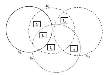
Figure 5.1: a WSN example composed of four sensors  $s_1$ ,  $s_2$ ,  $s_3$ ,  $s_4$ , distinguished by theirs sensing ranges represented by circles and targets  $t_1$ ,  $t_2$ ,  $t_3$ ,  $t_4$ ,  $t_5$ .
