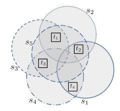
Figure 4.1: a WSN example composed of five sensors  $s_1$ ,  $s_2$ ,  $s_3$ ,  $s_4$ ,  $s_5$ , distinguished by theirs sensing ranges represented by circles and targets  $t_1$ ,  $t_2$ ,  $t_3$ ,  $t_4$ .
