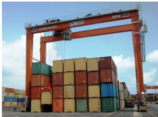
Figure 2.14: Rubber Tired Gantry Crane (RTG)
