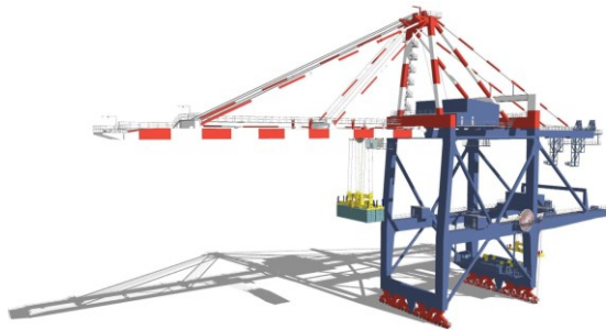
Figure 2.12a: Quay crane with dual trolley system
