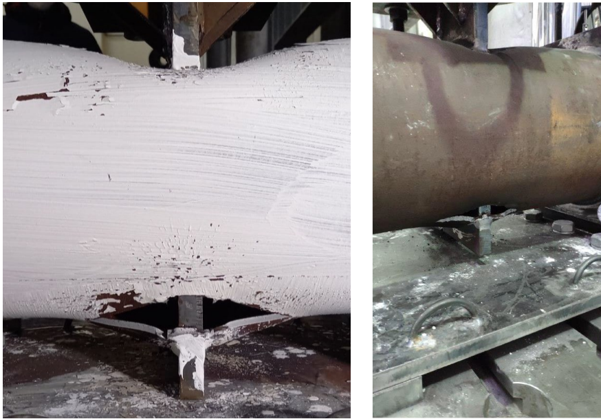
Figure 2.47 – Failure mode of Test 3: monotonic (left) and cyclic (right) loading
