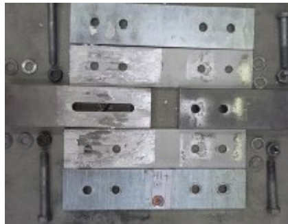
Figure 3.5 – Damage of the interfaces: M4 friction shims
