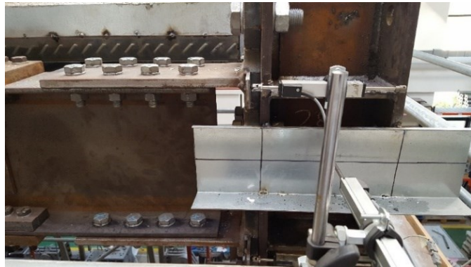
Figure 4.98 – Undamaged T-stub belonging to the second level at the end of Test 7
