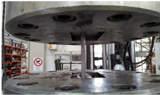
Monotonic test: stress-strain laws. f_y=368,4 MPa
