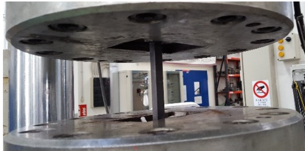
Monotonic test: stress-strain laws. f_y=346,6 MPa
