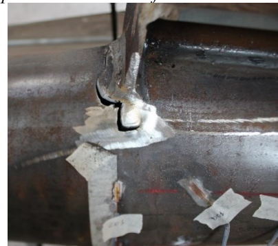
Failure mode of the specimen under monotonic loading
