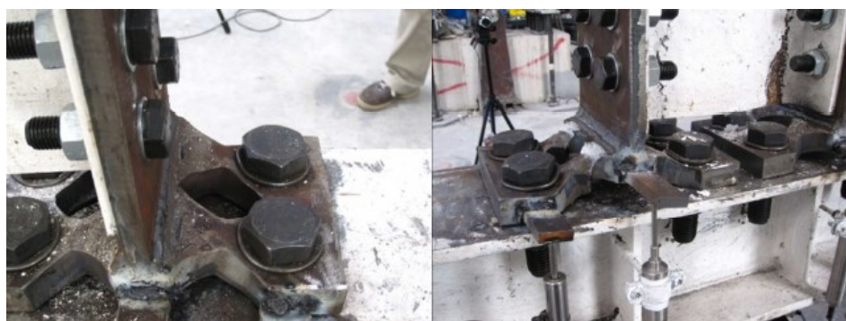
Figure 3.48 – Crack formation and propagation
