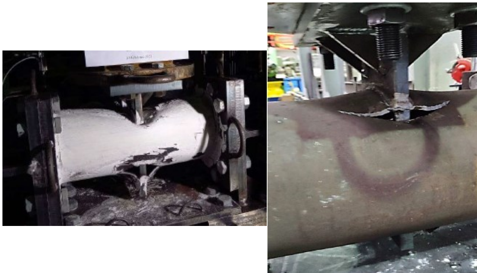
Figure 2.46 – Failure mode of Test 2: monotonic (left) and cyclic (right) loading
