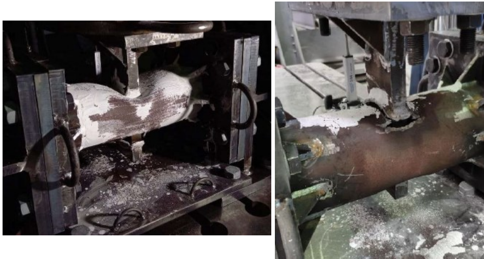
Figure 2.45 – Failure mode of Test 1: monotonic (left) and cyclic (right) loading
