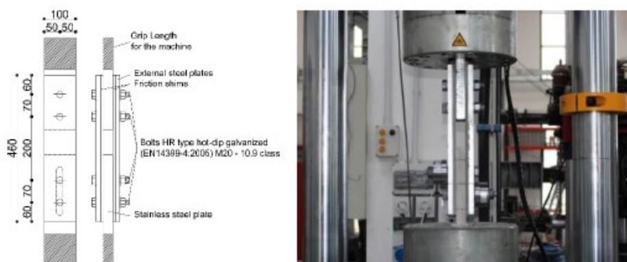
Figure 3.2 – Typical layout of a specimen (left); specimen in the testing machine (right)
