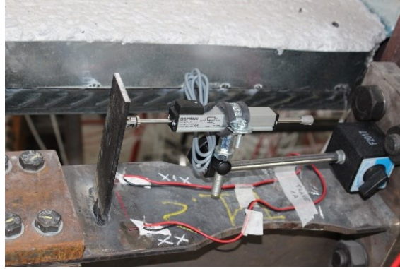
Figure 4.31 – Strain gauges on beams
