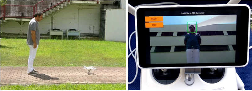
Figure 3.4: (Left) The drone stands by until a face is detected in the camera. (Right) The drone starting to take off when is detected a face.
