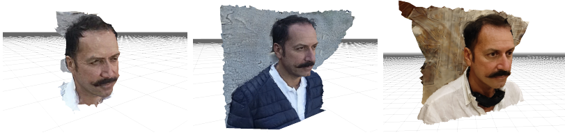
Figure 3.5: 3D reconstruction of half body left and center with FHD and C4K resolution from drone and right with FHD resolution from mobile device.
