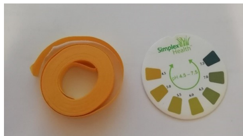
Figure 4.12: On the left a pH test strip, and on the right the colour references with associated pH level.
