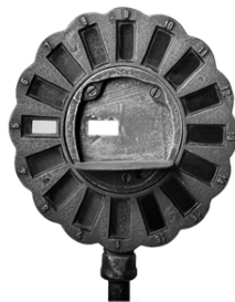
Figure 4.1: An example of the Lovibond Comparator.
