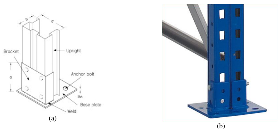
Figure 1.4: Schematic representation of a base-plate connection (a) (reproduced from [43]); and a detailed view of the footplate bolted to the upright.(b) (reproduced from systemsdesignuk.com ).
