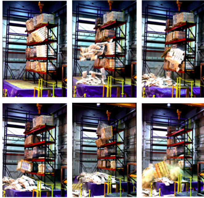
Figure 2.2: Shake table tests on non-isolated steel storage pallet racks [68]
