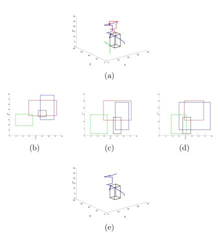
Figure 4.7 An overview of the method. (a) a query box and three trajectories; (b), (c), (d): the projections of trajectories' MBRs on the coordinate planes; (e) the final result of our method, after the application of the clipping algorithm on the blu and red trajectories.
