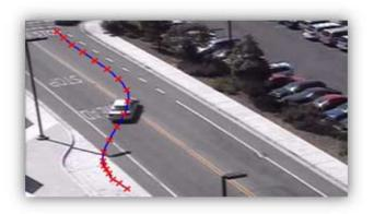
Figure 2.3 A vehicle with anomalous trajectory.
