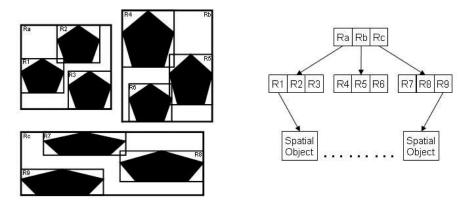
Figure 4.1 The structure of an R-Tree [MNPT05].
