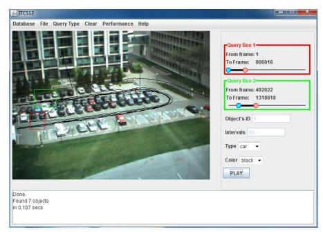
Figure 5.4 The Graphical user Interface designed for the Traffic Analysis Application.
